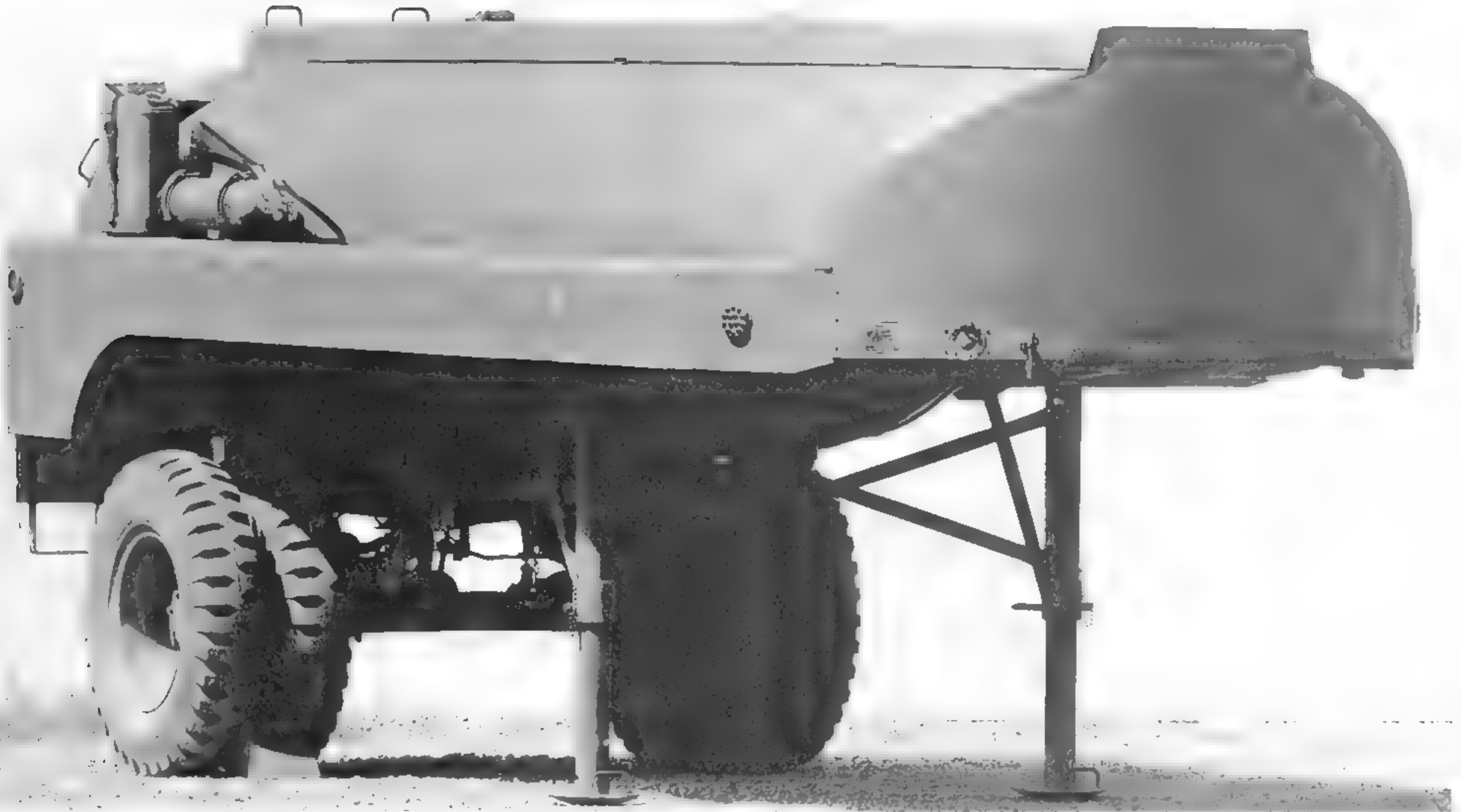
The wide stance of the landing legs provided for the G-678 series is apparent in this photograph taken at the Studebaker Proving Ground in 1944. Notice the fire extinguisher carried on the side of the trailer — crucial on fuel trailers such as this. (U.S. Army photo)
